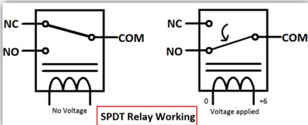
When there is no voltage applied to the coil, COM (common) is connected to NC (normally closed contact). When there is some voltage applied to the coil, the electromagnetic field produced. Which attract the Armature (lever connected to spring), and COM and NO (normally open contact) gets connected, which allow larger current to flow. Relays are available in many ratings, here we used 6V operating voltage relay, which allow 7A-250VAC current to flow.
