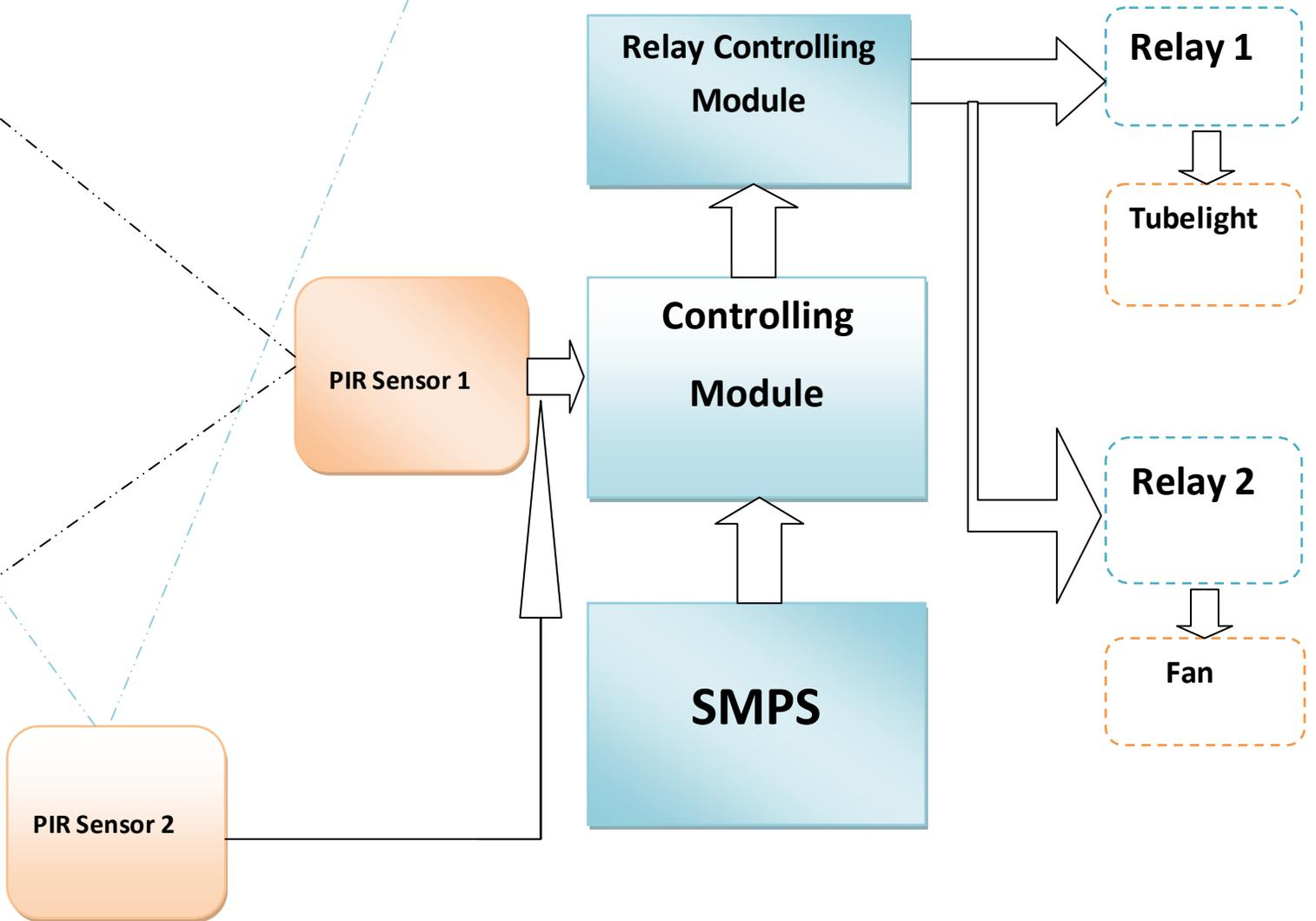
**In Principal's cabin we built the logic of two sensors. Because there was one error obtained of movement of person. Sometimes sensor could not detect the vertical movement. So we built the logic of two sensors one was at one for horizontal movement and one for vertical movement and it works successfully.**
